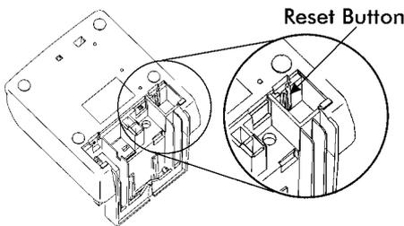
The RESET Button (which is long) is located in the right lower corner on the bottom of the clock.
