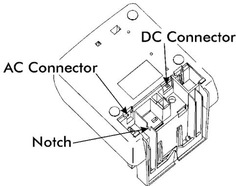
If you are using the DC power cord, locate the rubber grommet on the power cord and install the grommet into the notch in the housing. The power cord will exit the clock through the opening on the bottom. Refer to page 15 for more information about using the DC power cord.
