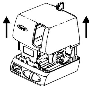
3. Remove the spacer between the Ribbon Cartridge and the Printer Carriage.
