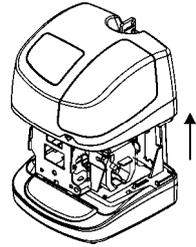
The Amano PIX-55 clock pictured to the right, shows a typical layout with the ribbon cartridge installed in the cradle.
