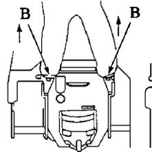
**Step 3.** While holding the release tabs in an upward position, grasp the tab on the ribbon cassette, and pull the ribbon cassette out of the cradle (see figure).
