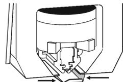
**Step 5.** Turn the knob on the cassette clockwise one turn to take up any slack in the ribbon (see figure).
