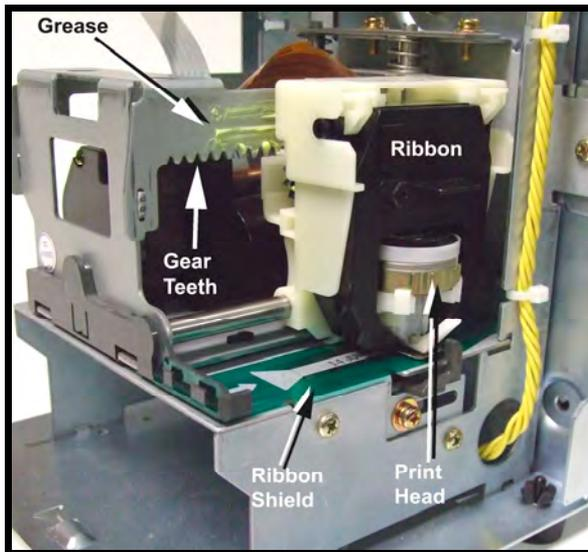
*Figure: Ribbon Carriage Grease*
