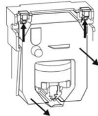
**Step 4.** Insert a new ribbon and be sure to mount it between the ribbon guide and the printer head as illustrated (see figure and arrows).
