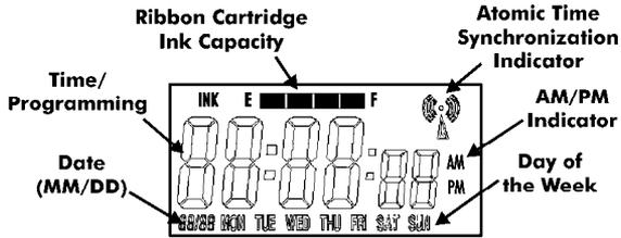
The LCD Display contains an Ink Capacity gauge. This gauge indicates the amount of ink remaining in the ribbon cartridge using four bar segments, from E (Empty) to F (Full).
