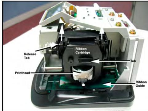
**Step 2.** Pull the two release tabs ("B") upward, and hold with index and middle fingers (see figure).
